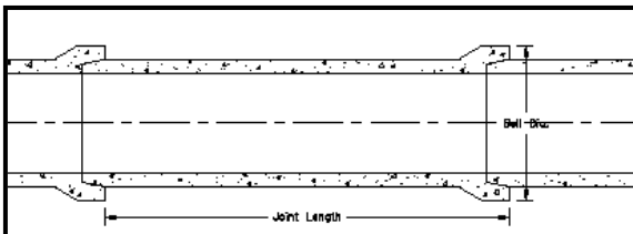
Typical Concrete Pipe Configuration
